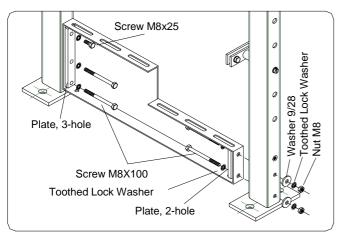
The screws M8x25 and 3hole plates aren't needed for 1and 2-row racks.
