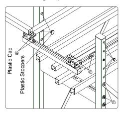
Pre-assemble holder. To this end use bolt M8x20 toothed lock washer and anchor plate.
