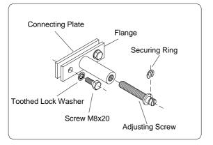
Insert telescopes in the stands from the inner side. Then secure with a securing ring.
