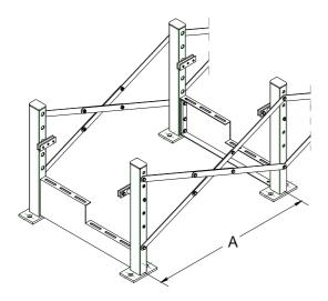
Place uprights in a vertical position and mount the brace according to distance A between the uprights, as defined in the enclosed diagram, and the respective distances  $A_1$ ,  $A_2$ ,  $A_3$ ... and so on.
