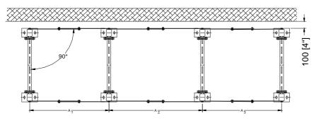
The gap between the rack and the wall or other appliances in the room must be at least 100 mm [4"].
