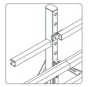
Insert upper lengthways rails and screw down tightly at intersections.
