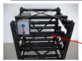
Insert the L-Profiles in the front of the rack. Put on the bracing in front and on the top of the rack.
